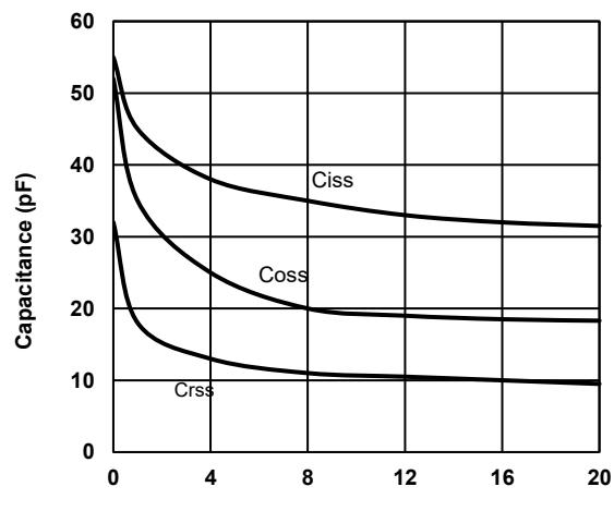
Fig6. Typical Capacitance Vs. Drain-Source
