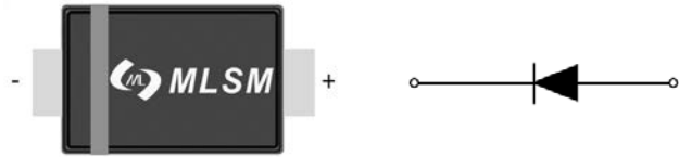
SOD-123FL top view
