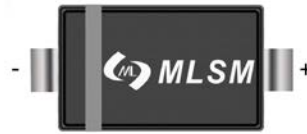
SOD-123 top view
